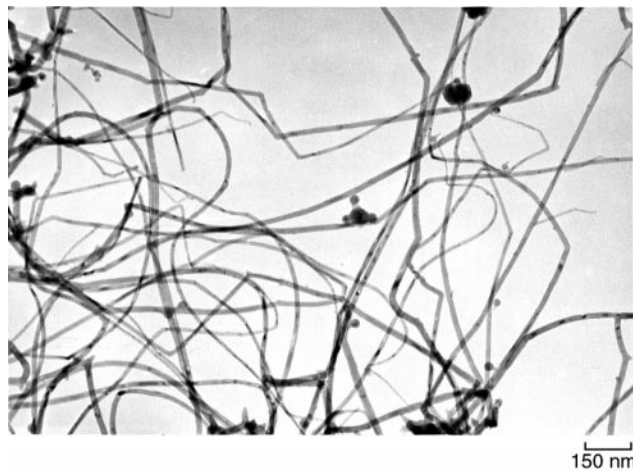
Fig. 1 Condensate obtained from the vapours liberated by a \text{Li}_2\text{SiO}_3/\text{Si}/\text{SiO}_2 mixture in Ar at 1800^\circ\text{C} .
